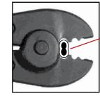
4.00mm Crimp Sleeve, Aligned Correctly
